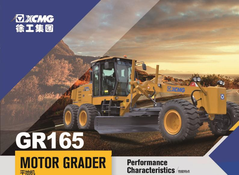
The motor grader is mainly used for ground leveling, ditching, slope scraping, bulldozing, scarification, snow removal for large areas such as highway, airports, farmlands etc. It is the necessary construction machinery for national defense construction, mine construction, urban and rural road construction and water conservancy construction, farmland improvement and so on.
